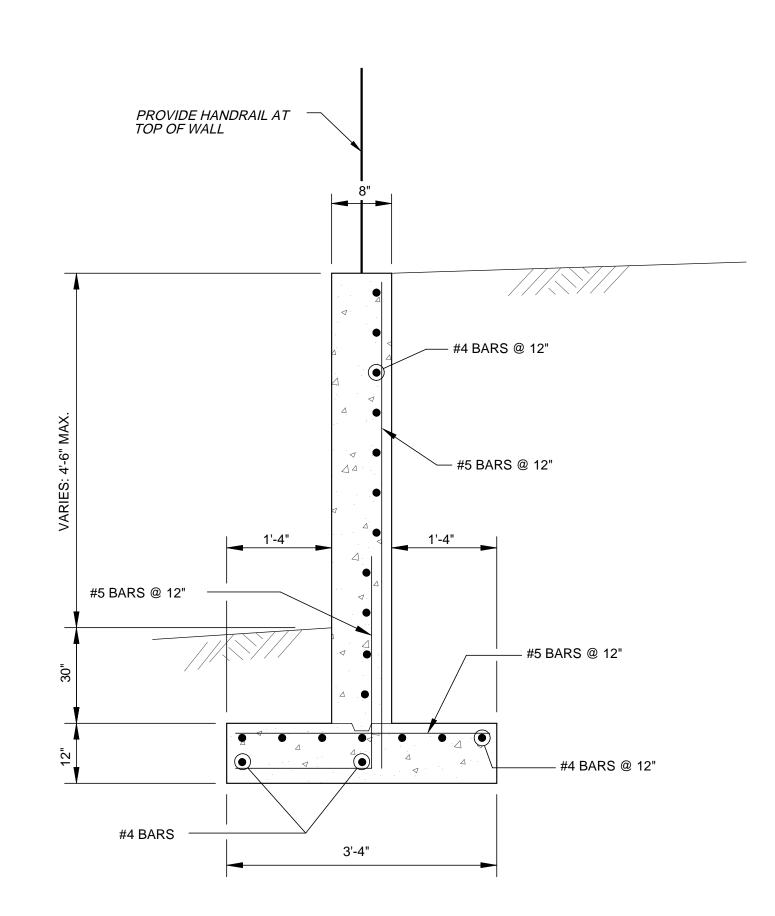
CONCRETE RETAINING WALL DETAIL
