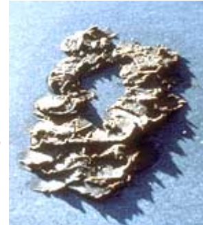
Removing felt-tipped marker graffiti with poultice.
