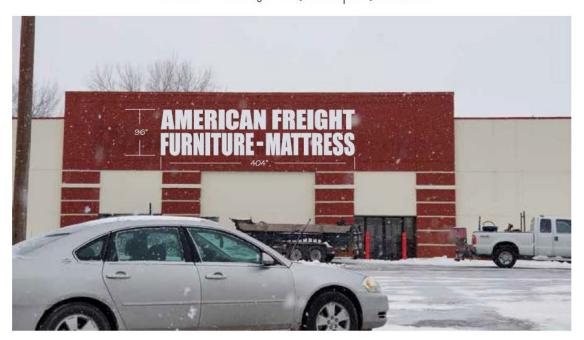
QUANTITY 1 SET AS SHOWN OF DIMENSIONAL CHANNEL LETTERS LETTERS TO BE CONSTRUCTED AND FORMED OF ALUMINUM EXTRUSION LETTERS / LOGO CAN BE INTERNALLY LIT OR LIT BY EXTERNAL LIGHT BARS CURRENTLY ON THE BUILDING.
