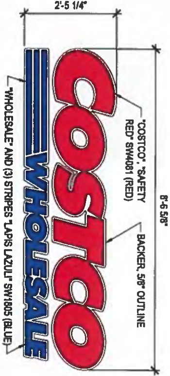
2 NORTH & SOUTH ELEVATIONS SCALE: 1/4" = 1'-0"
